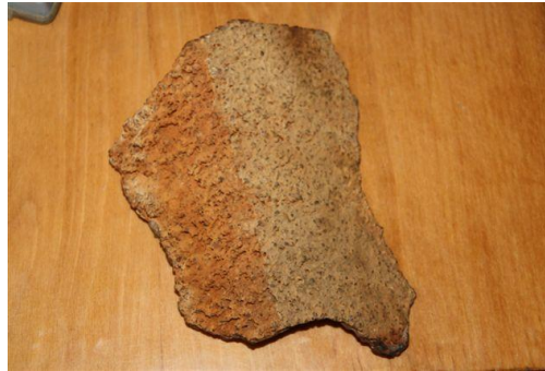
8.) accumulation in pipes, chamber etc.
